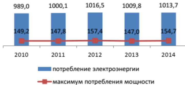
Electric Power Consumption in 2010-2015, kWh bn, and Peak Consumption for the Russian UES, MW thousand 3
